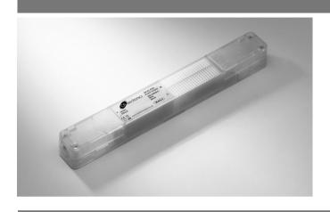
The DA-SL-PSU is an SELV 16VDC power supply primarily designed for DALI. The unit has an integral LED that is visible through the front window to indicate that the output voltage is healthy.
